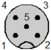
Figure 7: Contact configuration M12 plug
