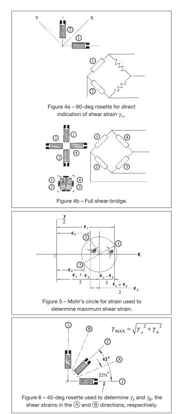
**Plane-Shear Measurement with Strain Gages**
