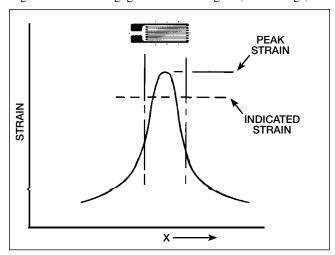
strain over the area covered by the grid. Since the average of any nonuniform strain distribution is always less than the maximum, a strain gage which is noticeably larger than the maximum strain region will indicate a strain magnitude that is too low. The sketch above illustrates a representative strain distribution in the vicinity of a stress concentration, and demonstrates the error in strain indicated by a gage which is too long with respect to the zone of peak strain.
