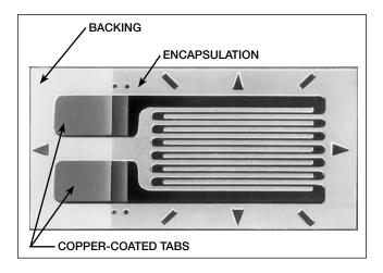
The C2A Series strain gages have been a popular choice in particular for field applications where time is of the essence. The C2A Series gages are a laminated polyimide-encapsulated A-alloy gage with 10 feet of pre-attached vinyl cable which helps to save time during the gage installation, whether in the lab or in the field.
