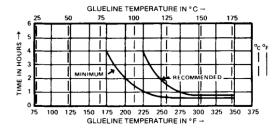
**M-Bond 610:** Cure at temperature for time period specified by graph below.
