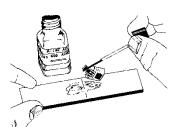
Now, by lifting at a shallow angle, peel back one end of the taped assembly so as to raise both gage and terminal. By curling this mylar tape back upon itself, it will remain in position, ready to be accurately repositioned after application of adhesive.
