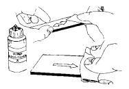
Preliminary dry abrading with 220- or 320-grit silicon-carbide paper is generally required if there is any surface scale or oxide. Final abrading is done by using 320- or 400-grit silicon-carbide paper on surfaces thoroughly wetted with M-Prep Conditioner A; this is followed by wiping dry with a gauze sponge.
