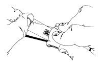
Immediately rotate the tape to approximately a 30-degree angle so that the gage is bridged over the installation area. While holding the tape slightly taut, slowly and firmly make a single wiping stroke over the gage/tape assembly with a piece of gauze bringing the gage back down over the alignment marks on the specimen. Use a firm pressure with your fingers when wiping over the gage. A very thin, uniform layer of adhesive is desired for optimum bond performance.
