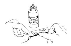
Now apply a liberal amount of M-Prep Neutralizer 5A and scrub with a cotton-tipped applicator. With a single, slow wiping motion of a gauze sponge, carefully dry this surface. Do not wipe back and forth because this may allow contaminants to be redeposited.
