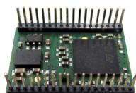
GSV-6CPU: 4V supply, output: 0...3V; CAN, UART, 6x ADC
