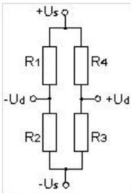
The external active resistors R3 and R4 are connected to
