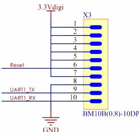
Figure 3: Terminal assignment of the configuration interface
