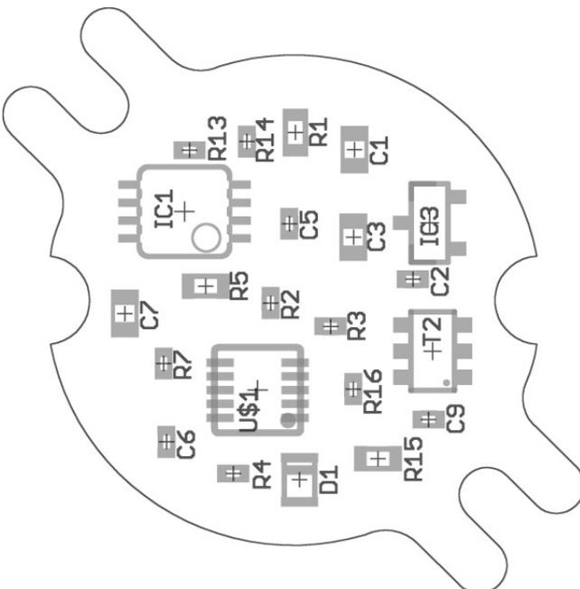
For an input sensitivity of about 2 mV/V, R5 is doubled.
