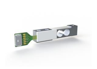
The KD60a force sensor is the successor to the KD60 force sensor. It also has the geometry of a miniature load cell and is attached on one side via the through holes. The force is introduced into the M5 thread. The force is introduced parallel when loaded. The force sensor tolerates displacements of the force introduction and transverse forces due to its double-beam design.
