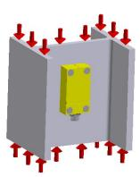
The full pressure strength of the magnets is only achieved on a flat surface. If there are small surface irregularities, air gaps occur between the magnet and the component meaning that the pressure strength is potentially insufficient to compress the strain gauge and the seal. Therefore please check whether the pressure strength of the integrated magnets is sufficient before applying the adhesive. For series DA68e, the following should be observed in particular:
